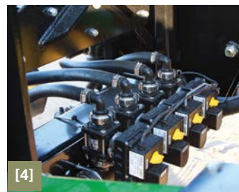
[1] Rubber torsion boom suspension [2] Custom tank [3] Center pivot boom [4] Boom valves [5] Welded steel frame
