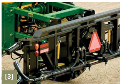
[1] Rubber torsion boom suspension [2] Custom tank [3] Center pivot boom [4] Boom valves [5] Welded steel frame
